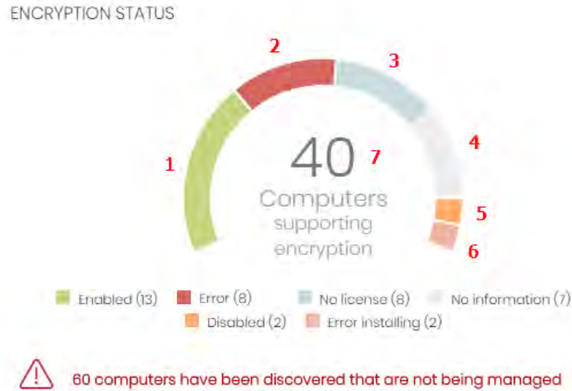
Figure 16.2: Hotspots in the Encryption Status panel
